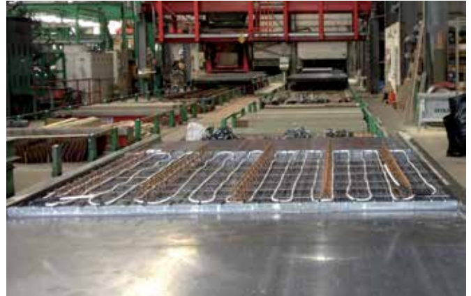
View of the prefabricated filigree slab in the manufacturing site.
