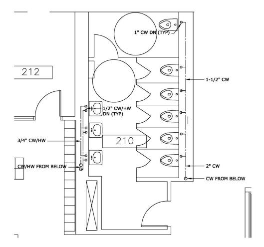
Figure 2- Restroom 210 Isometric
