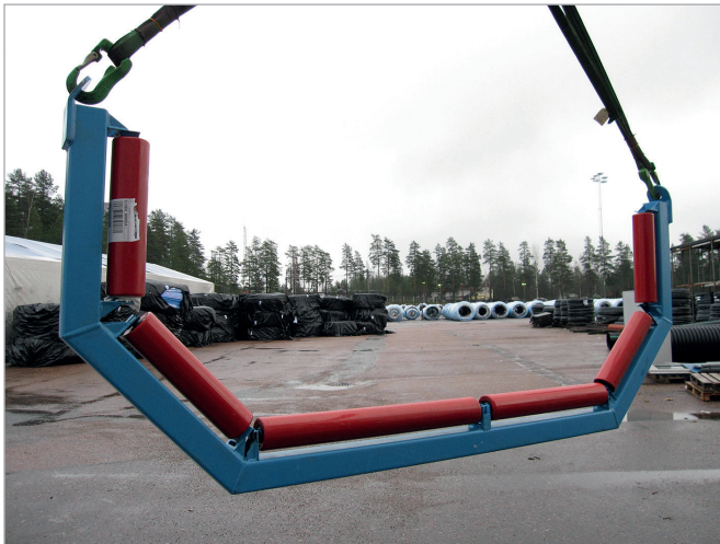
Solid holders and the roller guide with three sides ensure maximum safety when laying heavy Ecoflex coils up to 650 kg.
