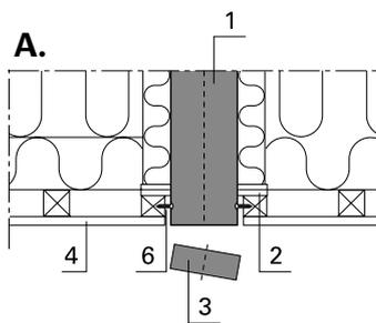
**A.** Cut the duct to the level of the finished roofing, using, for example, a saw with fine tooth pitching, or duct cutting pliers. Secure the duct from inside with two mounting screws.
