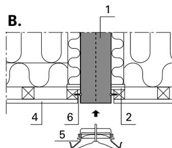
**B.** Insert the valve into the duct. The valve locks on the duct and no additional mounting procedures are required. Please note: If the roof valve is connected not to the duct but to a duct component, the valve seal must be replaced with a special seal ordered separately. For further information, please contact EH-muovi.
