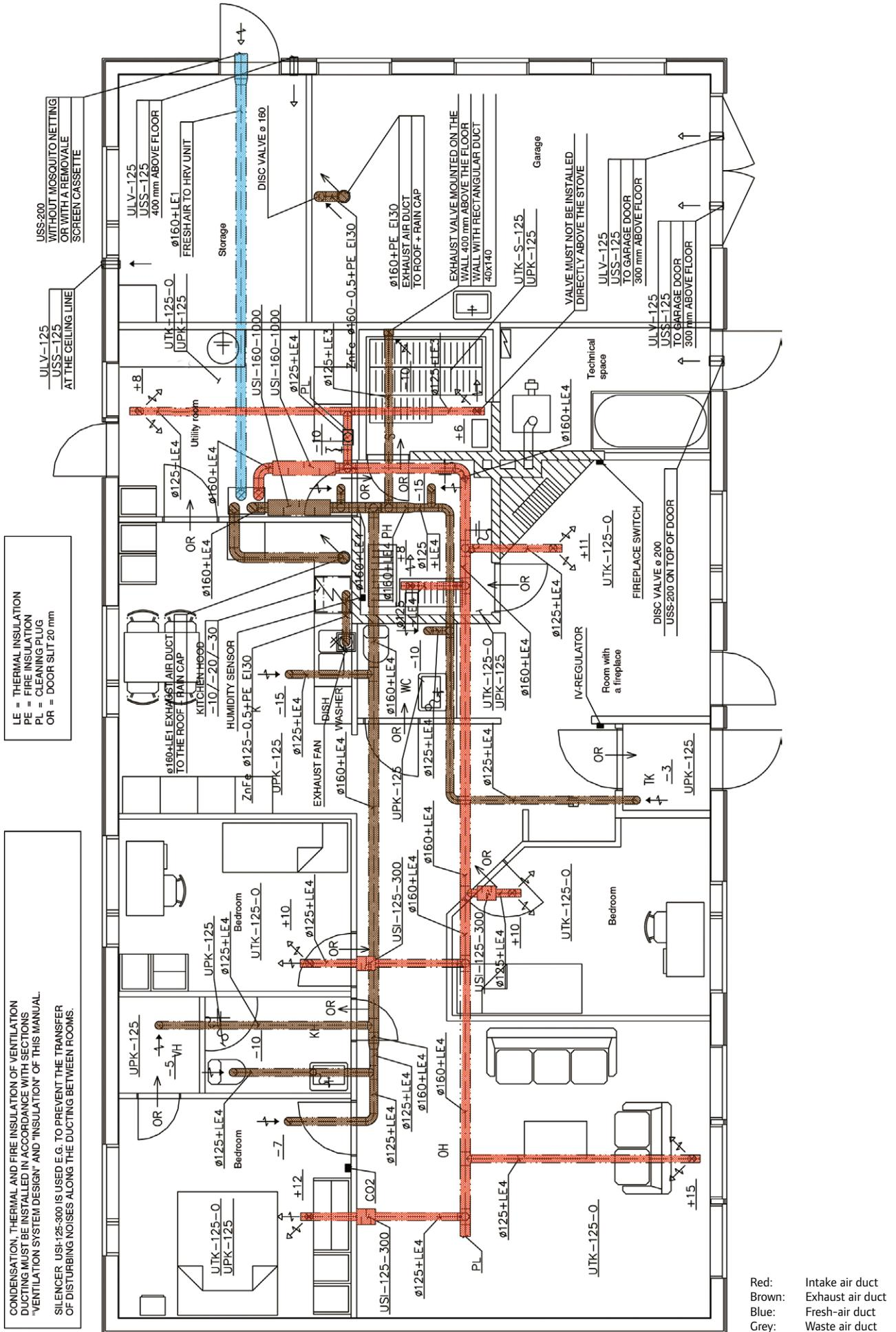
Example of a ventilation system design for a detached house. Bill of materials on the following page.
