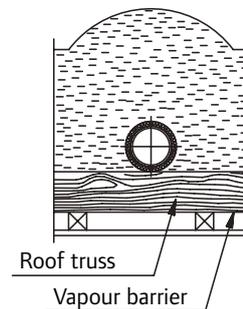
Duct in loose mineral wool or similar. PE expanded plastic insulation, LE 4, or 50 mm mineral wool, LE3, is used. Installation of a duct embedded in loose mineral wool or similar is not recommended.
