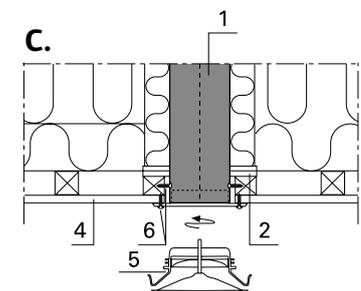
**C. The supply and exhaust valves of saunas,** intended for ceiling mounting, are equipped with mounting frames that are secured to the ceiling structure with screws. Attach the valve to the frame by rotating it. Ceiling-mounted frames installed above the sauna stove must always be secured with screws.
