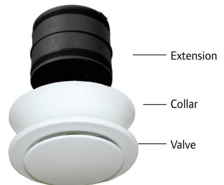
**E. The wall-mounted valve** is installed by pushing it into the duct, which is cut to the level of the wall surface. The valve cover may be removed by twisting it with a screwdriver. The base is equipped with holes for the mounting screws.
