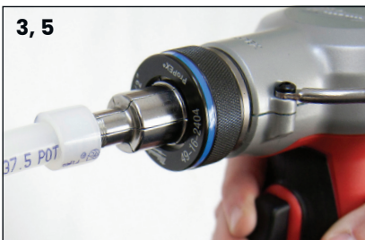
Figure 3-3: Expansion with Milwaukee M12, M12 FUEL, M18, and M18 FUEL 2" ProPEX Expansion Tools
