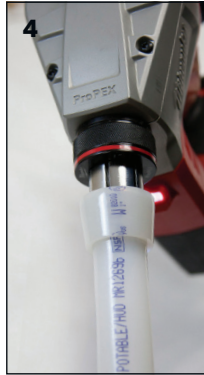
Figure 3-8: Expansion with Milwaukee M18 ProPEX Expansion Tool
