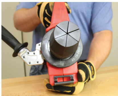
Figure 3-12: Correct Expansion Head Alignment
