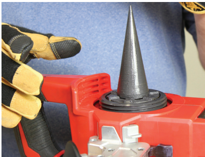
Figure 3-9: FORCE LOGIC Expansion Head Installation
