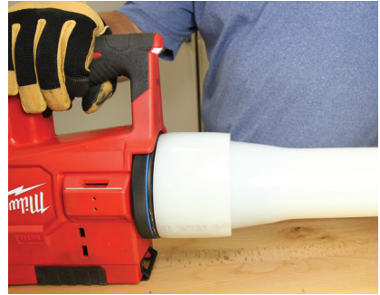
Figure 3-17: Expand to Shoulder
