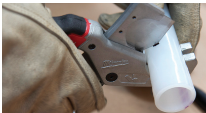
Figure 3-28: Cut Pipe at Marking
