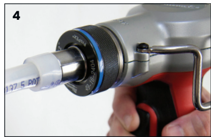
Figure 3-3: Expansion with Milwaukee M12, M12 FUEL, M18, and M18 FUEL 2" ProPEX Expansion Tools
