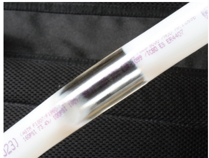
Figure C-1: Reforming Kinked Piping
