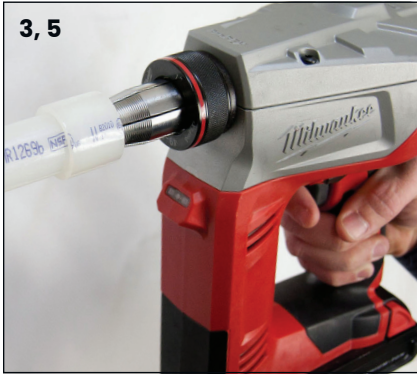
Figure 3-8: Expansion with Milwaukee M18 ProPEX Expansion Tool
