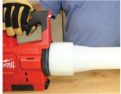
Figure 3-17: Expand to Shoulder
