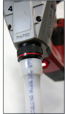
Figure 3-8: Expansion with Milwaukee M18 ProPEX Expansion Tool
