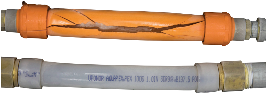
Figure C-2: CPVC vs. PEX Freeze Test
