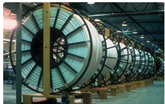
Wirbo-inPEX pipes can be made in lengths of up to thousands of metres. This reduces the need for fittings, simplifies installation and reduces costs.
