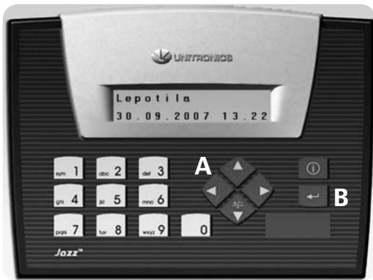
A Arrow keys used to move in the software submenus B Enter key used to accept choices
