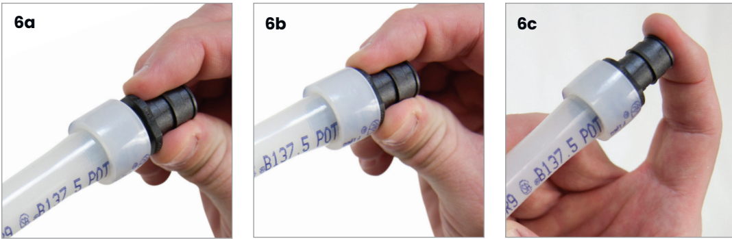
Figure 2-5: Inserting ProPEX fitting into 1/2" Uponor PEX piping
