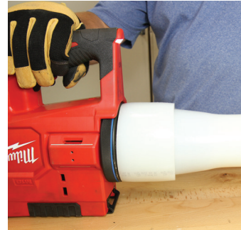
Figure 2-18: Expand to shoulder
