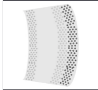
Figure 1-2: PEX-b (Silane) 65-70% crosslinked
