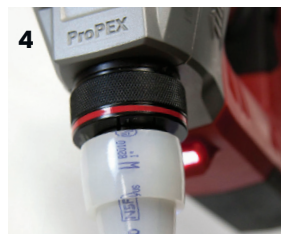
Figure 9: Expansion with Milwaukee M18 ProPEX Expansion Tool
