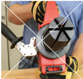
Figure 12: Incorrect expansion head “flowering”
