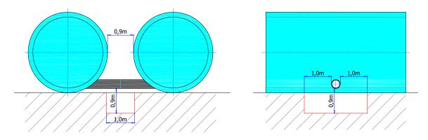
16. In the excavation, at the location where the welded joints of the tank body are to be made, the Principal shall make 0.9 m deep pit, as wide as the outside diameter of the tank + 0.9 m on each side of the installation pit and approximately 2 m long. Depending on the soil and water
