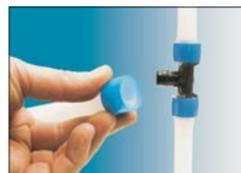
**Step 3. Enter the tube into the ring** keeping the edge lightly out (maximum 1 mm) of the tube. In case the ring has a top end and angle of entry, these two properties will facilitate the use and assembly of both tube and ring.
