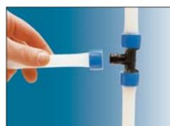
**Step 6. Carry out the joint:** keep the pipe in its place against the end of the fitting during 3 seconds. After this time the pipeline will have contracted on the fitting, and it is possible to make another joint. The joint can be made up under a minimum environment temperature of -15°C. It is possible to use the hand, the electric battery or the hydraulic expander.
