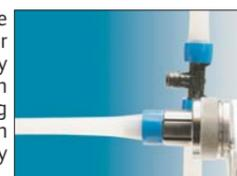
**Step 5. Last expansion:** when the pipe touches the end of the expander head, the last expansion must be done. If the joint is to be assembled in a difficult place, keep the pipe in its place against the end of the expander head during 3 seconds after the last expansion, before opening the arms of the expander tool. Finally, withdraw the expander.
