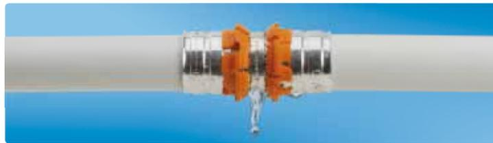
If a connection is still not pressed, this is shown up doubly when pressing. The coloured stop rings are still attached. Additionally the fitting is designed in such a way that during the pressure test water leaks out. Now simply press and the connection is permanently tight.
