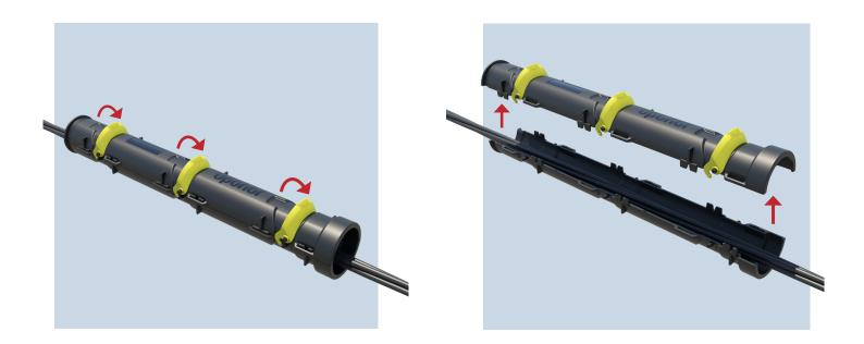
Disassembling the cable protector. Open the lock with your foot or hand. Lift the pipe half with locks straight upwards.
