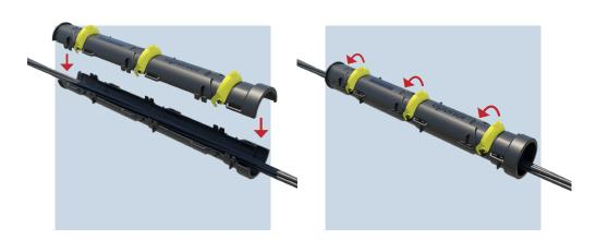
3. Place the pipe half with locks on top of the pipe half without locks.
