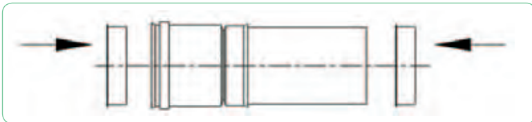
Figure 8.2.22. End plug installation.
