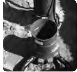
Clean Easy channels water to the distribution chamber, from where it is distributed to the land filter trench/infiltration system.
