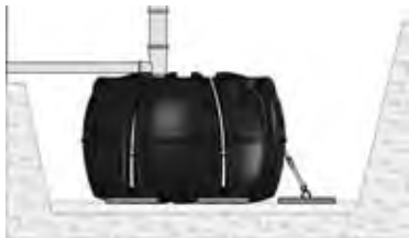
Anchoring with anchor plates.
