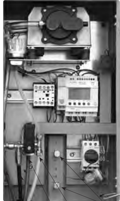
Connect the red hose here. Connect the black hose here. Connect the green hose here. Connect the yellow hose here. Mounting bolts.
