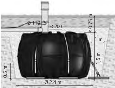
The low built holding tank from Uponor is easy to install.
