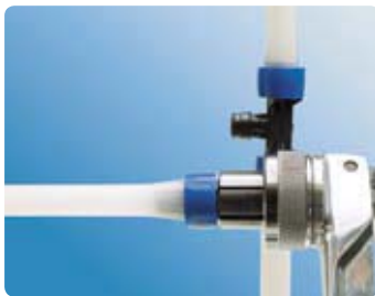
Widen the pipe end with the expander tool
