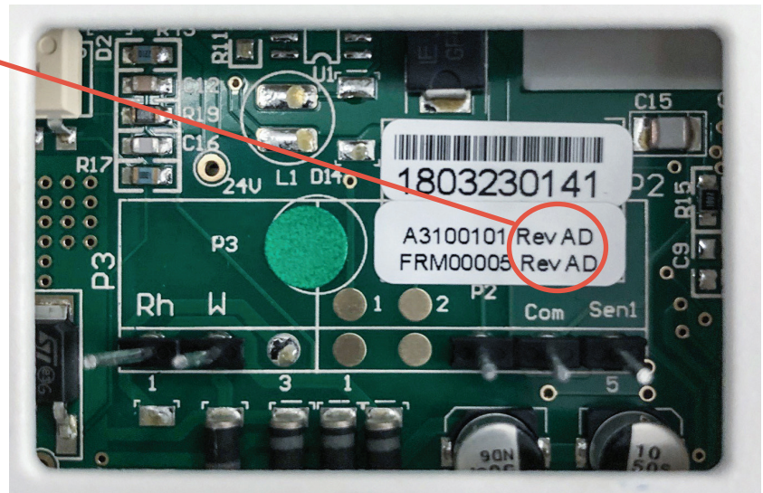
Figure 1: Circuit board sticker
