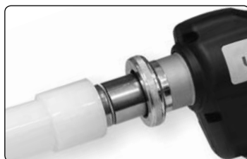
Figure 4-3: Slide Expander Head into Tubing
