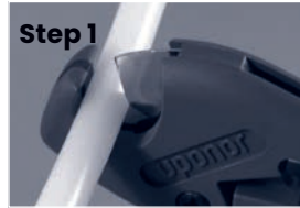
Figure 3: Square-cut the pipe
