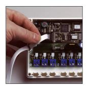
**2.** Fasten the actuator cables into the blue contacts.
