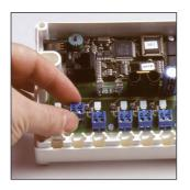
**5**. Connect the Programmer and Control Unit with the white cable supplied.
