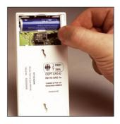
**9.** The thermostats are installed using the black cable supplied. Push the cable into the socket at the side of the Control Unit.
