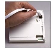
**3.** Using pliers, break-off the plastic where the cable will pass through the box
