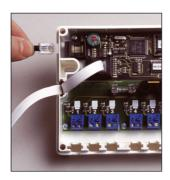
**12.** Select the channel to which the thermostat is to be assigned with the horizontal arrow keys and confirm with "OK". If the thermostat controls several channels repeat the programming by disconnecting the cable and connecting it again.
