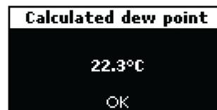
The screen displays the dew point calculated by the Climate Controller C-46.
