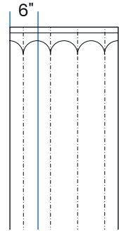
Figure 7: Cut 6" wide down entire length of panel
