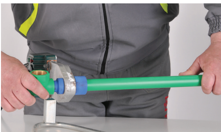
Figure 2-3: Heating the pipe and fitting
