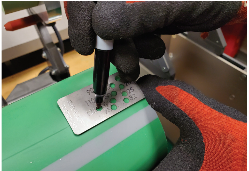
Figure 2-2: Mark weld depth
