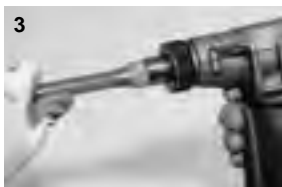
Figure 7: Expand the pipe and ring until it reaches the collar. Then complete a minimum of one more expansion.
