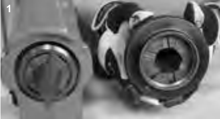
Figure 13: When installing 2"- 3" heads, ensure the cogs are aligned and engaged with the tool.
