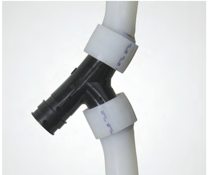
Figure 1-5: At approximately 2,900 lbs. of pull force
