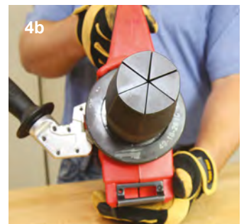
Correct expansion head alignment
