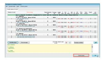
A dialog box appears for the design of floor heating/cooling regulation. In the list of manifolds, mark **manifold** and select **regulating system** and check the **required functions**. By means of *Set up regulation system for multiple manifolds*, the selected type of control can be set including the selected functions for other manifolds in the project.
