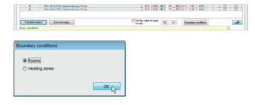
Within the boundary conditions of **rooms**, the maximum surface temperature and the minimum and maximum temperature gradient of living (LZ) and boundary (BZ) zone are entered. The program uses default values, each of which can be edited.
