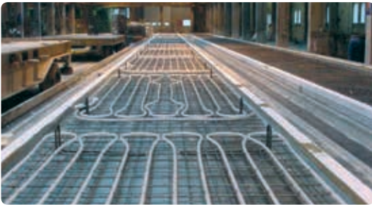
Uponor Contec modules incorporated into precast concrete slab
