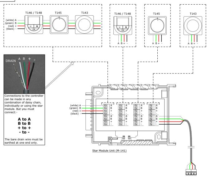
The Star Module must be either wired as shown into the Base Controller / Slave Module Unit or plugged into the end of them.
