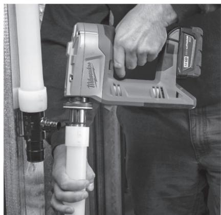
Figure 3-13 : Outil de dilatation Milwaukee M18 ProPEX
