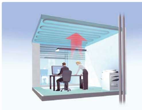
The cooled ceiling slab accumulates the thermal loads from the room or direct sunshine
