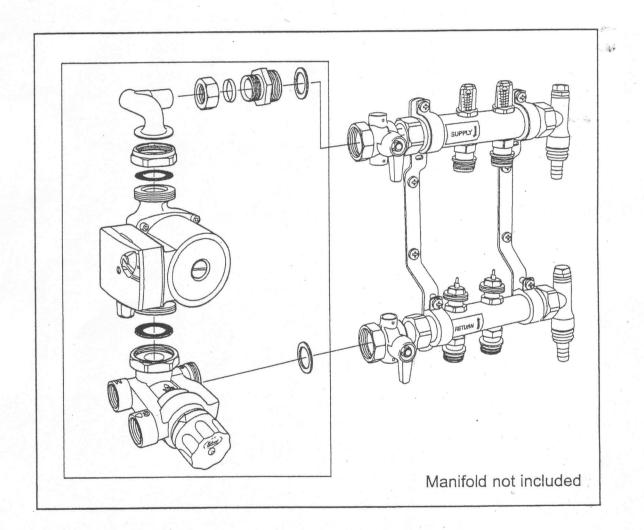
The Manifold Control Pack provides temperature controlled mixed water to an underfloor heating system with a heat output up to 14kW.
