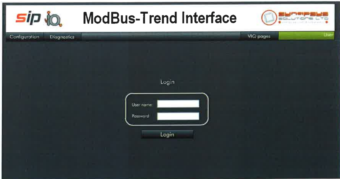
SIP Login Menu – Default user name is 'Admin' (capital 'A'), Password is 'password'
