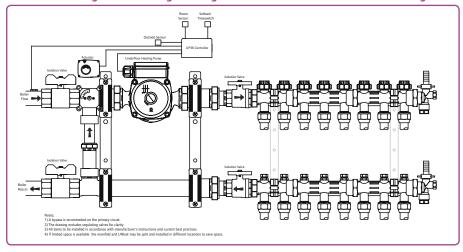
Electrical schematic drawing showing UNIset MIDI/MAXI wired for single zone control
