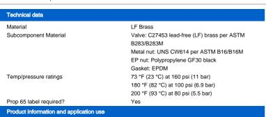
Use Uponor ProPEX® lead-free (LF) brass water meter service valves in all commercial submetering and residential water service inlets, outlets or both. The valves allow for a direct ASTM F1960 connection to water meters sized 5% to 1". Valve is sized for 3% or 1" Uponor AquaPEX® tubing. Product handle material is stainless steel.
